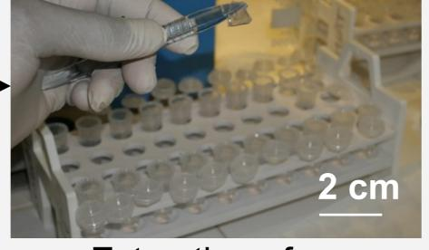
Extraction of resin binding gel from DGT
