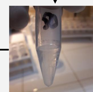
Elution of resin binding gel in HNO<sub>3</sub> 1M for 24 hrs
